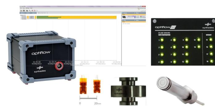
**OptiFlow** monitoring unit has 4 channels (which can be extended up to 40 e.g. **Optiflow32** version) for monitoring the resin arrival and temperature at 4 locations providing a certified resin arrival signal by monitoring the electrical resistance of the resin and a reliable temperature measurement based on RTD sensing.
