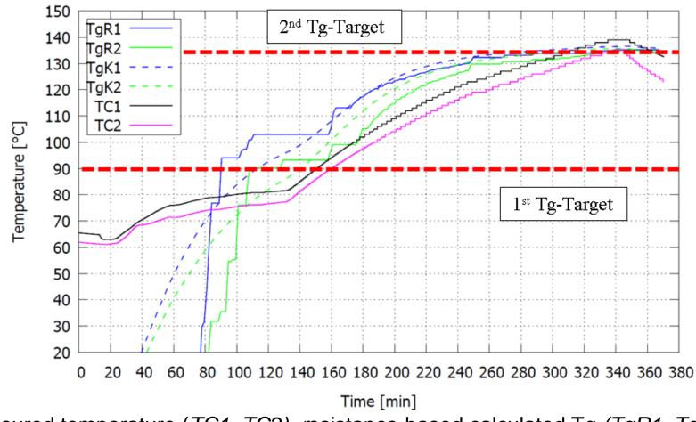
Measured temperature (*TC1, TC2*), *r*esistance-based calculated Tg (*TgR1, TgR2*) and the theoretical Tg (*TgK1, TgK2*) for the C1 and C2 sensors together with the Tg targets
