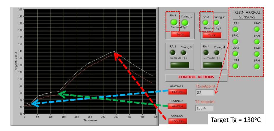
Real-time Tg calculation and demoulding decision based on targeted Tg (target Tg =  $130^{\circ}$ C)
