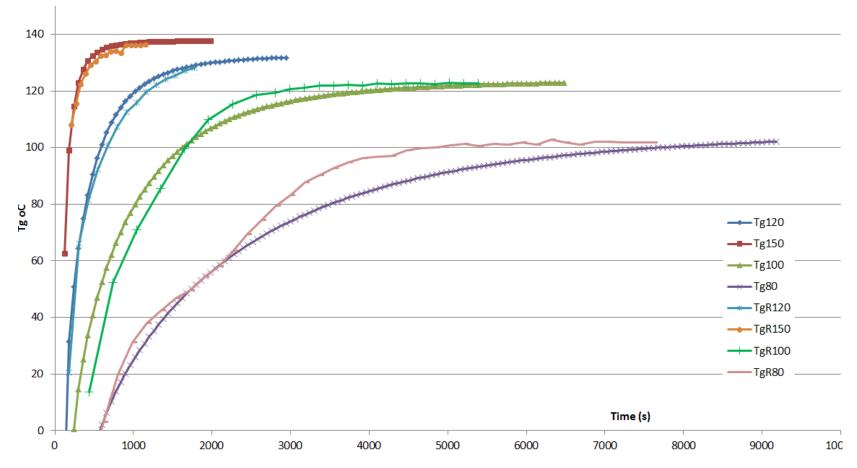
Tg prediction based on resistivity (TgR\*) and on kinetic models (Tg\*) for 4 isothermal cycles at 80°C, 100°C, 120°C and 150°C.
