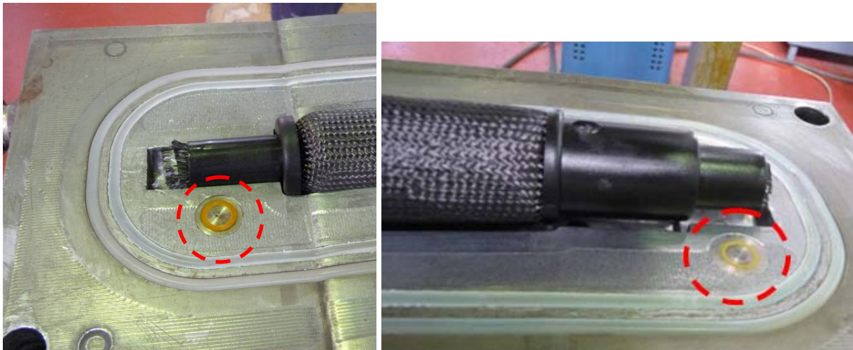
Fig.6. Flush mounted sensor at the cavity’s margin near the inlet (left) and outlet (right) gates.
