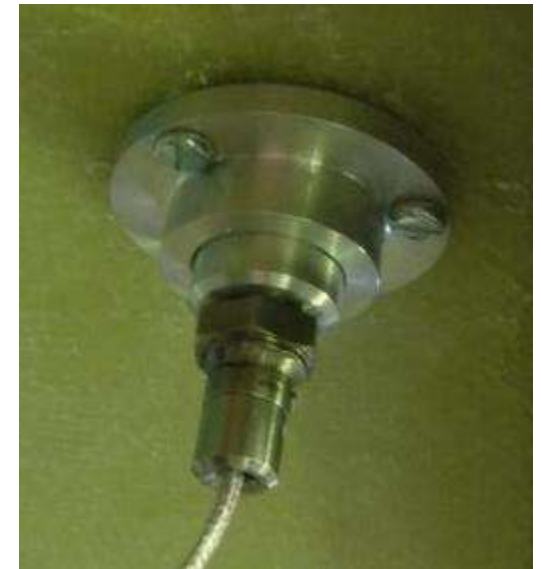
CUSTOM-MADE ADAPTOR FOR COMPOSITE TOOL
